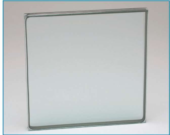
Sungate 400 glass is a highly transparent, low-e glass designed specifically for heating-dominated, northern climates. It is manufactured with an MSVD “soft coat” that helps buildings retain solar and furnace heat to reduce winter heat costs.
